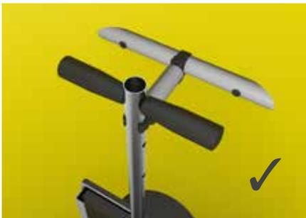
Remove the lifting bar with the handle and the throttle from the shaft. Disassemble the handle. Cut the lifting bar at the marked position (use a saw or angle grinder), remove edges. Reassemble the handle and insert the component into the shaft.
