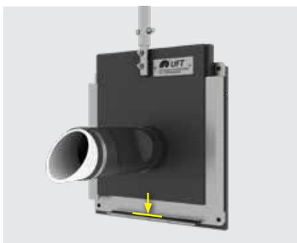
Afterwards, insert the tube throttle with the lifting bar into the shaft and insert the board into the guides of the stainless steel base plate. Make sure to insert the board down to the lowest stop edge of the stainless steel base plate.
