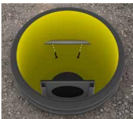
Position the fixture for the lifting bar vertically and centrally over the stainless steel base plate and screw directly into the shaft wall, no primary drilling required.
